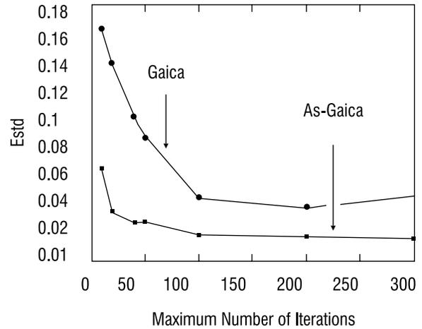
**Figure 5: Maximum number of iterations versus standard deviation of the error signal**
