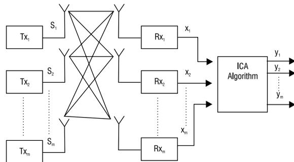
**Figure 1: Block diagram of ICA system model**
