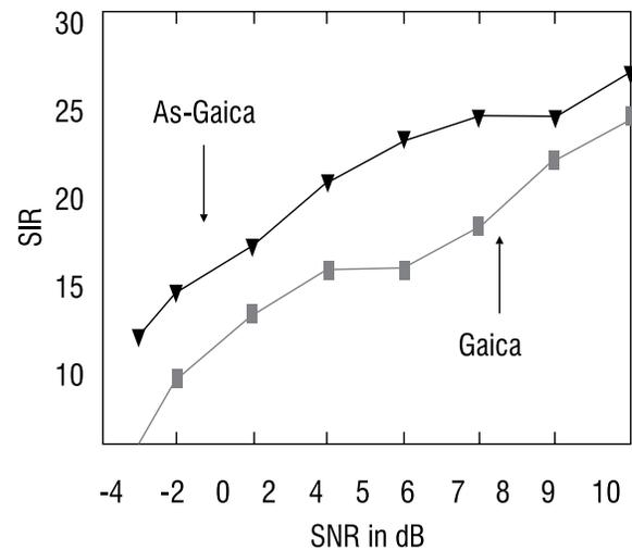
**Figure 6: SNR versus SIR in dB for the GAICA and AS-GAICA algorithms**
