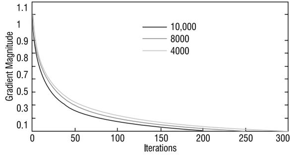
**Figure 7: Convergence characteristics of AS-GAICA algorithm for different size of input data block**
