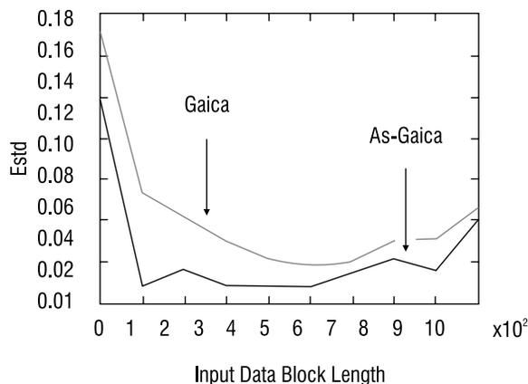
**Figure 4: Input data block length versus standard deviation of the error signal**
